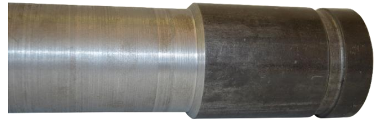
milled section of pipe
